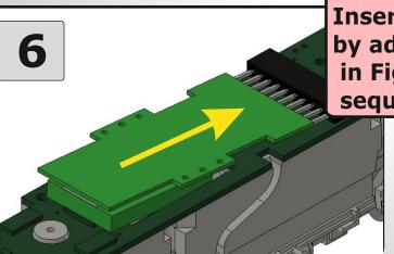
Insert the adapter into the main board by adopting the procedure shown in Figure 3, this time in reverse sequence.
